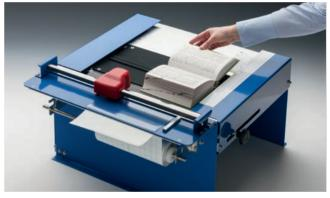
5. Please ensure that there is an overlap here, too, of 2 cm for the book cover. The distance between the edge and the head of the cutter should be about 2 cm. Open the book roughly at the middle and check the printed scale to see how much of the filmolux® film you will need to pull off the roll.
