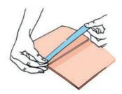
and then the other side to the opposite book page. Rub the strip firmly with a burnishing bone to achieve good adhesion. Cut off any overlaps with scissors. If repairing very thin paper or where text has to be covered, you can use filmoplast® P instead of filmoplast® P 90.
